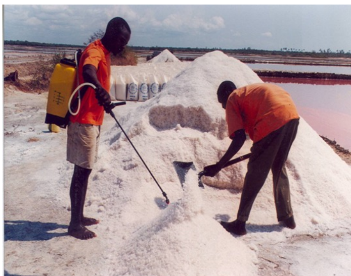
Iodation of salt using a knapsack sprayer
